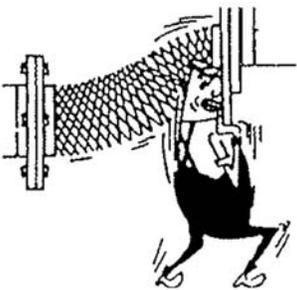
Don't force the connector into too much lateral offset as this puts it under extreme strain and in this position it cannot handle any other movement. And do not sharply bend the connector near the pipe end. The flange or fitting end must always remain perpendicular to the axis. If the piping meets at an angle, install the connector with a shallow curve along its entire length leaving a small straight section at each end.
