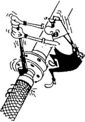
Don't impose torque or force rotate one end of the connector. This sets up residual torque stress in the connector which causes cracking of the corrugations or the fitting weld. On threaded connectors, use two wrenches to prevent torque stressing the connector and be sure to use the fitting end of the connector, do not apply to the braid collar.
