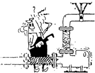
Anchor the piping close to the connector at the end opposite to the source of the vibration. Failure to anchor in such a manner will result in transmission and possible amplification of the vibration through the piping. Use hangers on all adjacent piping; do not let the connector support any weight except its own. The light wall is designed to contain internal pressure, not carry external loads.
