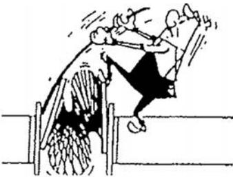
Don't compress or stretch a connector to make it fit. Compression stresses the corrugated element, slackens the braid pressure restrainer, reduces further compressive movement and generally results in early failure. Stretching places excessive stresses on the braid and braid collar and can result in early rupture.
